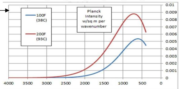
These black body graphs show emissions at typical temperatures of the black foam board at the back of the boxes. Emissions at these wave numbers are incident on the covering materials. The red transmission spectra give the percent of the incident emissions that get through.
