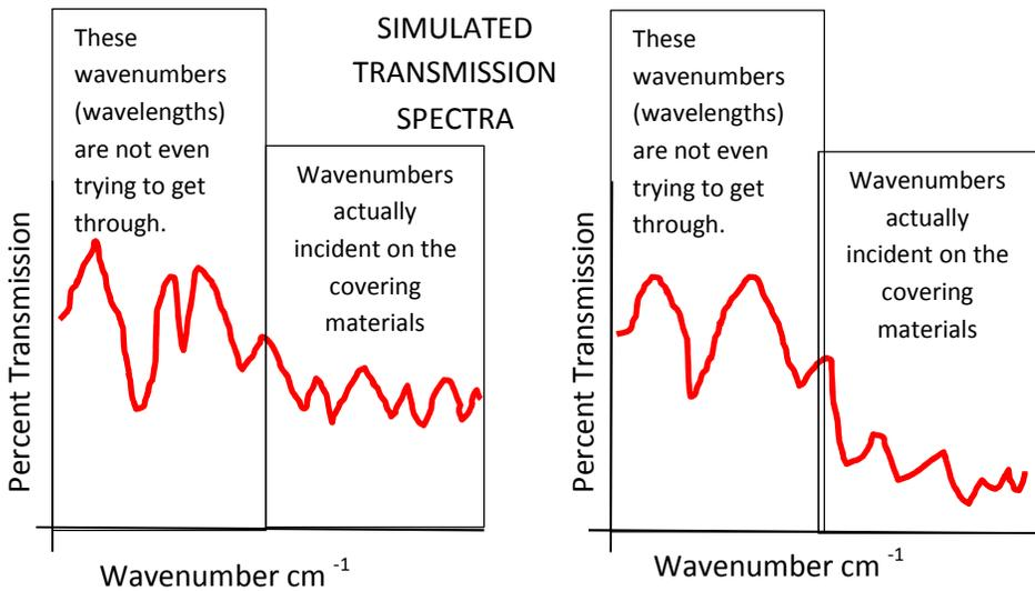
8. It was possible to qualitatively notice which covering material was transmitting more and which less. Here the right-hand material is transmitting less and thus trapping more infrared at least in the wavenumber range actually used. (Panels 6, 8)
