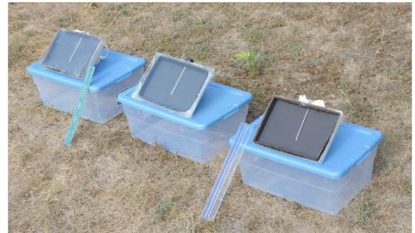
Boxes used here for the first set of trials and platforms for holding them. Notice the control box with no cover (extreme right). The 30-cm rulers show the scale. Sometimes paper stuffing was necessary to keep the thermometers touching the bottom. They measured 3 cm x 16 cm x 24 cm. Notice the drought conditions, which at least gave me a lot of days of weather that was good for this project.
