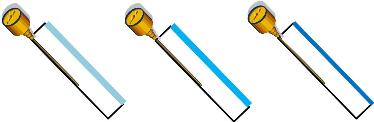
6 I stuck a cooking thermometer in each box to measure the temperature near the black material lining the bottom (black foam board). The thermometers themselves reside inside of a reflective metal tube (I took one apart and checked). They are not in direct sunlight. The tubes are designed to be stuck into a hunk of meat being cooked, but they served the purpose here. (I'm retired. I use what I find.)
